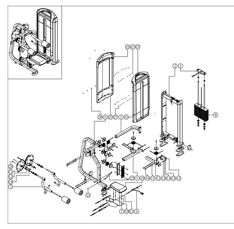
FF05 Lateral raise explosive view Note: spare parts and fasteners are not listed on the form.
